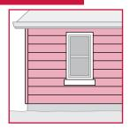
Install non-combustible siding (stucco, metal, stone, cement fibre board).
